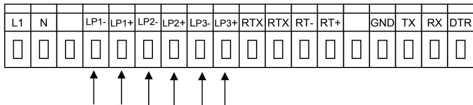
The incoming pulses are recorded in the load profile (see *Load profile for meters at the pulse inputs*, page 23).
