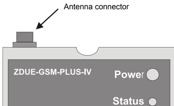
The antenna is connected to the FME antenna socket.
