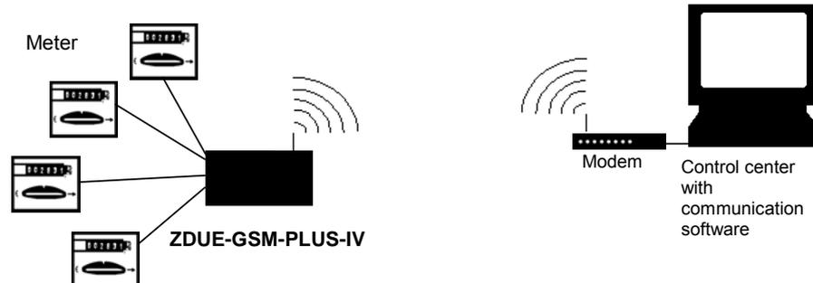
The ZDUE-GSM-PLUS-IV has the following interfaces for the connection of meters: CL1, RS-232, RS-485 (or M-Bus) and 3 pulse inputs. The maximum permissible number of meters can be connected simultaneously to each of the interfaces.
