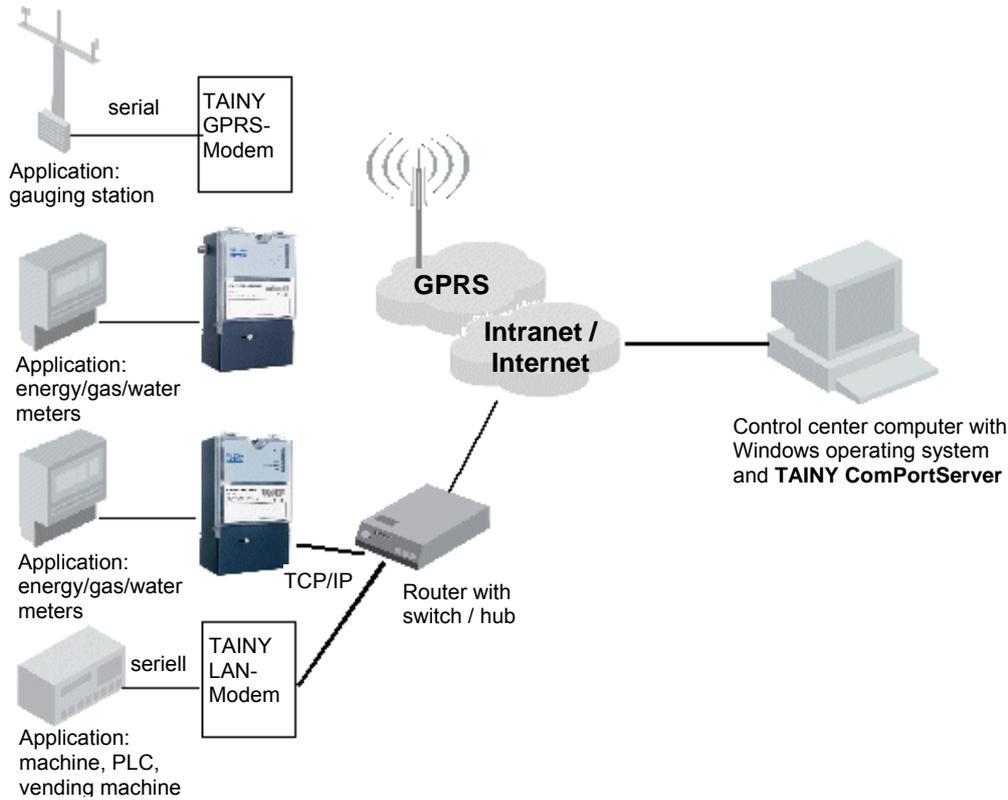
Any application connected to the ZDUE-GPRS-PLUS-IV/ZDUE-LAN-PLUS-IV can communicate with the control centre – and vice versa. The TCP/IP connection is routed via the Intranet and/or Internet.
