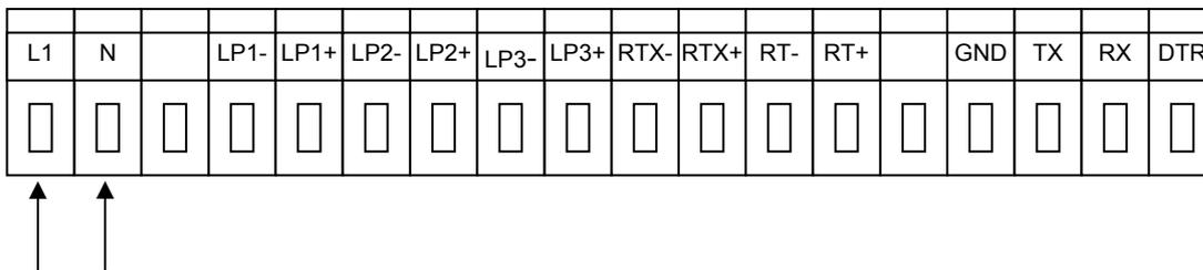
The ZDUE-GSM-PLUS-IV can be operated with either alternating current or direct current. The device complies with Protection Class 2. The supply of the interfaces is galvanically separated from the electronics.
