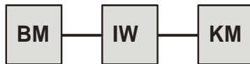
Figure 10 Connection variant between base module (BM), pulse emitting module (IW) and communication module (KM).
