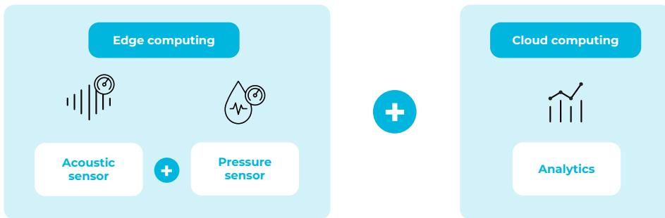
The primary goal of all utilities is to reduce, detect, and accurately locate these types of losses to ensure efficient water management and sustainability. These objectives are achieved by integrating analytical solutions into innovative meters with pressure and acoustic (vibration) sensors, using a patented solution from Sotto®.
